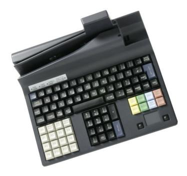
The swipe and park banking keyboard from Devlin Electronics has been specifically designed for retail banking applications. The KMX-093-300 features a hybrid reader mechanism with an integrated 'swipe and park' device. The keyboard is 'future proofed' allowing an easy migration and a cost effective path for banks changing, or upgrading, their teller platform, especially when implementing smart cards.
