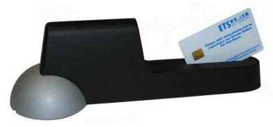
The eKrypto™ PCI Swipe & Park Reader Horizontal has an integrated combined hybrid ISO 7816 & EMV2000 approved Smart Card Reader (SCR) & 3 Track Magnetic Card Reader (MCR) in a Swipe & Park format for convenience. The hybrid reader approach is very effective for speeding up transaction times when both Smart and Magnetic Cards are still in circulation.
