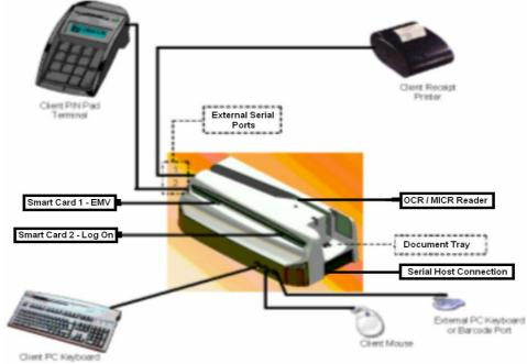
The BIRD is essentially a Serial device integrating a cheque reader, two smart card readers and two free external Serial ports.
